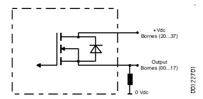
**Protections:** The outputs are grouped by 4 channels. They are protected against overload or short circuit using a thermal device. The protection acts on the group that presents the failure, deactivating the outputs and sending a signal to the software.. If the user do not configure this option the module will try to retrieve the outputs again. This characteristic avoid the use of a fuse base..
