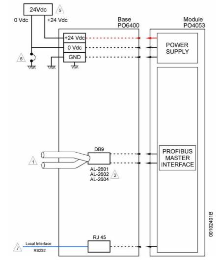
The diagram shows 24V power supply and PROFIBUS cable wiring with PO4053 module installed on PO6400 base. MU209903 - PO4053 Utilization Manual must be consulted for greater details.
