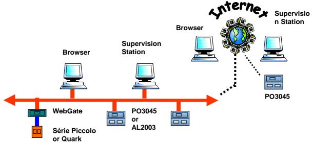
As shown oh the diagram, all Altus controllers may now communicate through TCP/IP networks. Through the WebGate, old and brand new controllers from AL-600, Quark, Piccolo and AL-2003 Series also may take advantage of the Internet.
