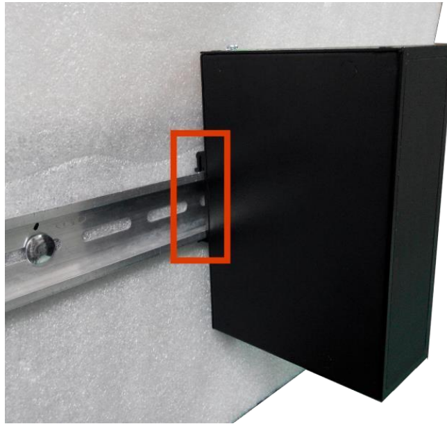
Figure 32: Stabilize the switch on the DIN rail
