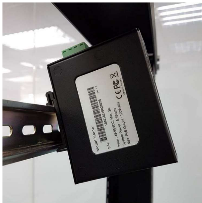
Figure 11: Insert the Media Converter into the DIN rail
