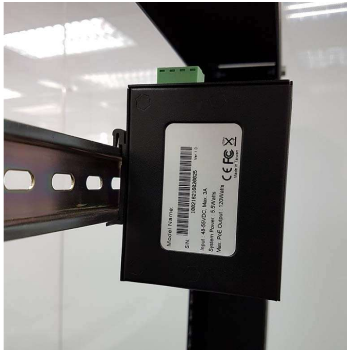
Figure 12: Stabilize the Media Converter on the DIN rail
