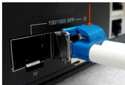
Figure 25: Removing the LC Connector
