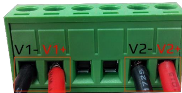
Figure 27: Power Terminal Block
