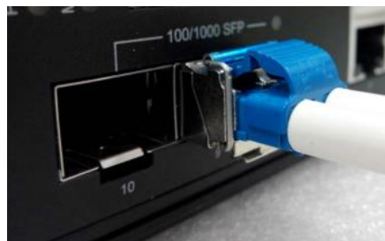
Figure 24: LC connector for the transceiver
