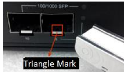
Figure 22: Transceiver for the SFP module
