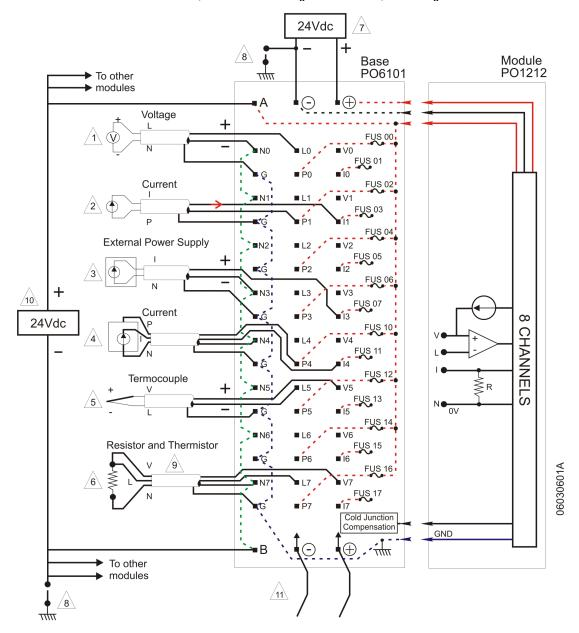
The diagram below shows the PO1212 electrical connection with the analog bases PO6104 or PO6004. For the base PO6005 the fuses, indicated in the diagram as FUS 0x, must be ignored.
