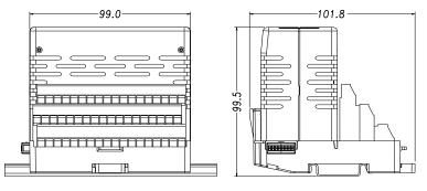
Here is the PO1212 module assembled in a PO6101, PO6104 or PO6151 fused terminal base in DIN TS35 rails.
