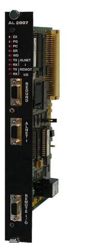
The hot-standby redundancy is used in applications that require high degree of availability, where two complete AL-2004 PLCs are connected to the same remote I/O system.
