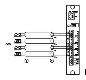
To connect a voltage output, the points V and AGND must be used.
