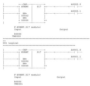
The logic number 002 shows how toread module inputs. Direct reading is possible because the module was declared in the bus as AL-3139. Input points reading is independent of the configuration.
