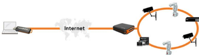
With its factory default settings, the Lock is connected to the Internet via its WAN port or a USB modem that can be connected to the USB port of the Lock. In this mode, the Lock creates its own protected local network for the connected devices. Only devices that are connected to the Lock by cable are accessible with the Key.
