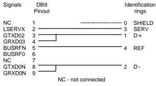
The cable shield is not connected to the DB9 connector. It's connected only to the AL-2600 SHIELD pin.
