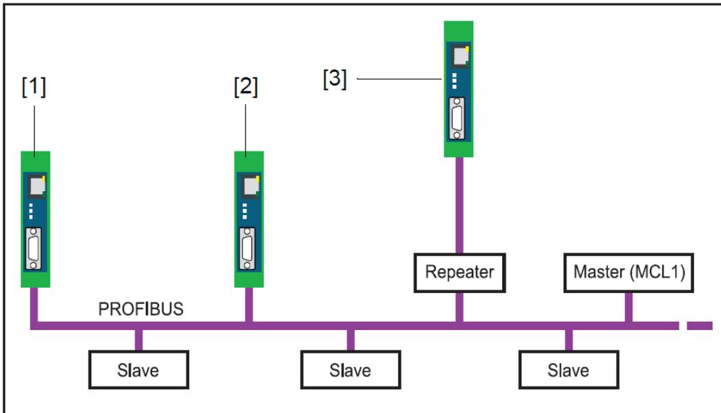
The previous diagram shows the connection possibilities on a PROFIBUS network:
