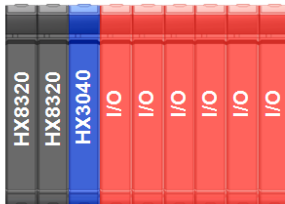
Figure 1: Power Supply Redundancy
