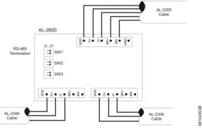
The 6<sup>th</sup> position is reserved for a earth ground connection, but only one of the AL-2600s in the bus must have this connection done, to avoid ground loop currents. The terminal marked as ground must be connected to the installation ground with a 1 to  $1.5 \text{ mm}^2$  gauge.
