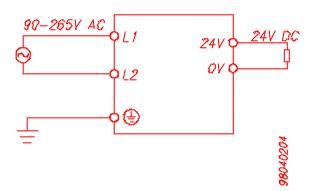
Conect the load to the terminals 24V and 0V and the mains to the terminals L1 (phase) and L2 (neuter) and protection ground according to figure shown above.
