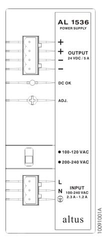
The output connection is composed of a 4-position female terminal, with conductors mounted by means of bolts. The identification of the assembly positions is shown in the following table:
