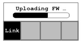
After uploading, select File/Reconstruct Source in H-Designer to display the Open dialog. Open the uploaded application file (\*.C64 or \*.AA6). The application screen will be displayed on the PC monitor. Finally, select File/Save As to save the application as a \*.V6F file. Thus a source file can serve the purposes of maintenance and modification.
