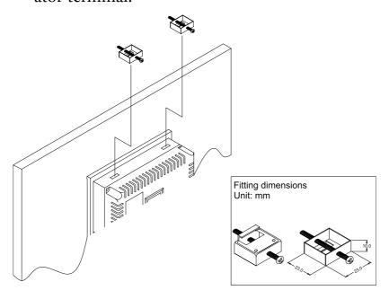
3. The operator terminal is to be installed within the angle of 0 to 135  $^{\circ}$  as shown below.
