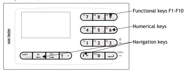
The Functional or Auxiliary Keys F1- F10 can be defined in H-Designer. They can, for example, be used to set a controller bit or register, to change a screen or to display a password table. Please see the H-Designer User's Manual for details.
