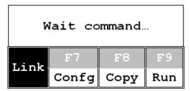
A command that is highlighted with black background on the screen is currently being executed by the operator terminal. Commands with gray background (e.g. F7, F8 ...) can be executed if the associated function keys are pressed. The functions of the commands are briefly explained below:
