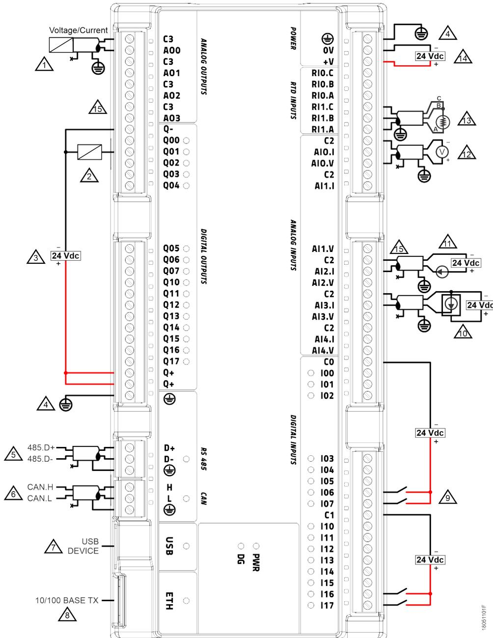
Figure 1: XP3xx Electrical Installation Diagram
