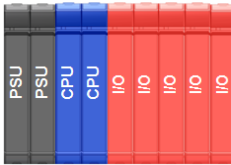
Figure 10: CPU Redundancy and Power Supply Module
