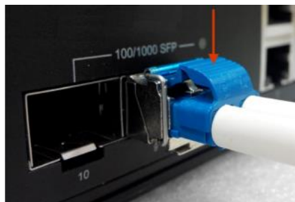
Figure 23: Removing the LC Connector
