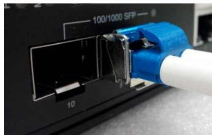
Figure 22: LC connector for the transceiver
