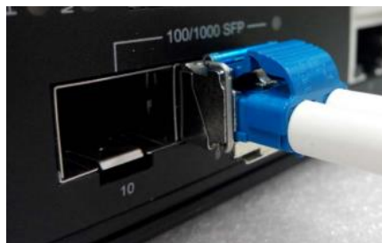
Figure 24: LC connector for the transceiver
