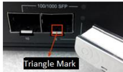
Figure 22: Transceiver for the SFP module
