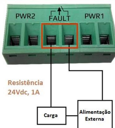
Figura 30: Conectando o Contato de Alarme Fault nos Switches ET2-0602-M, ET2-1600, ET2-0702-SFP and PT2-0500-24
