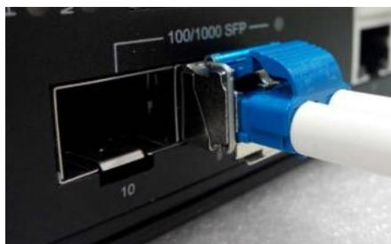
Figura 22: Conector LC para o transceptor
