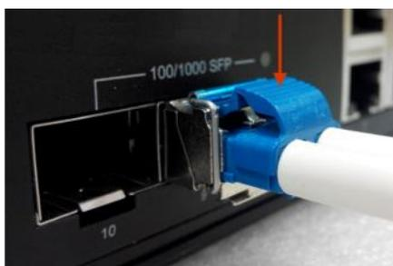
Figura 23: Remover o Conector LC
