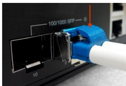
Figura 23: Remover o Conector LC
