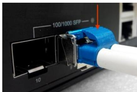
Figura 25: Remover o Conector LC
