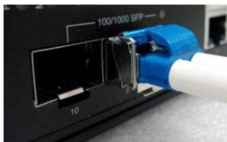
Figura 24: Conector LC para o transceptor
