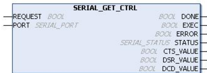
Figure 137: Block Used to Visualize the Control Signals
