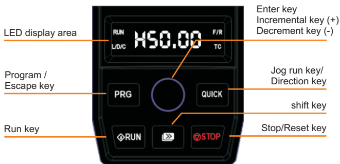
Figure 4-1 Built in LED digital display operation panel (standard configuration, non removable)
