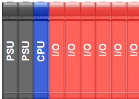
Figure 1: Power Supply Redundancy
