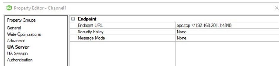
Figure 3-2. Example of Endpoint URL in client Kepware®
