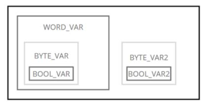
We can observe that in this context, BYTE\_VAR and BOOL\_VAR are contained within WORD\_VAR (which will have its bytes reversed in the architecture change), therefore, they are subject to endianism.
